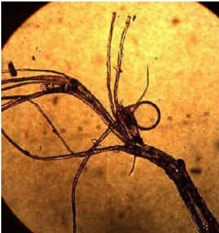
Figure 12: Heavily encrusted fibers from the outside of Raes #14 (400X) mounted in water 13: The same fibers shown in figure 12 mounted in 6N HCl. Notice the bright yellow color
